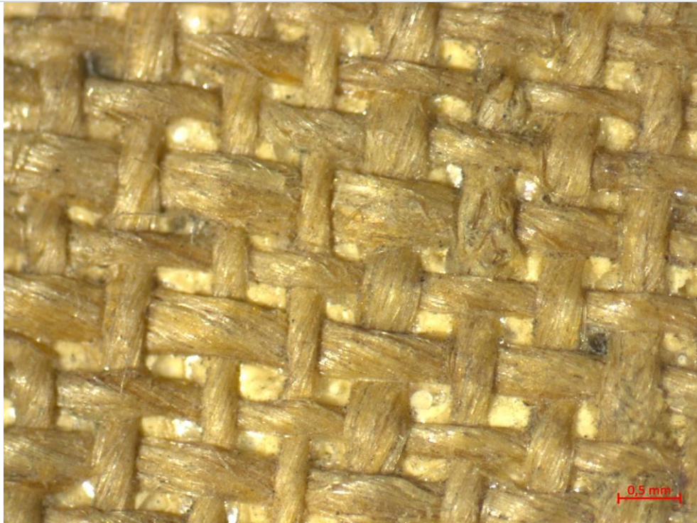
Figure 3: Still Life with Coffee Pot , microscopic photograph, x 20, reverse, incident light. The type of textile weave is a tabby weave with one thread in both directions.
